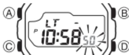
1. In the Timekeeping Mode, hold down (A) until the seconds start to flash, which indicates the setting screen.
