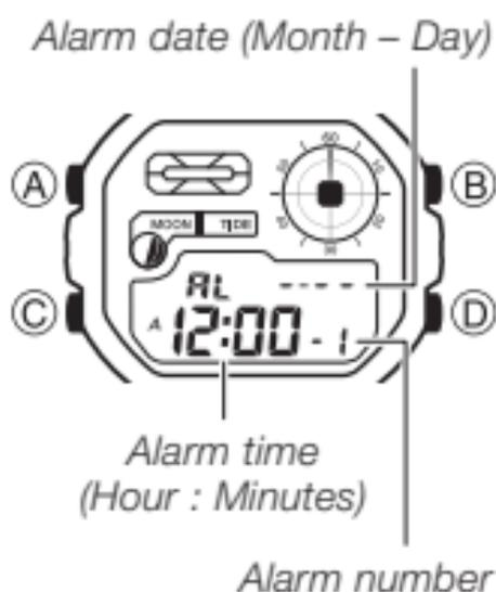
You can set up to three independent multi-function alarms with hour, minutes, month, and day. When an alarm is turned on, the alarm tone sounds when the alarm time is reached. One of the alarms has a snooze feature.
