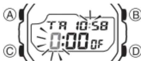
1. While the countdown start time is on the display in the Timer Mode, hold down (A) until the hour setting of the countdown start time starts to flash, which indicates the setting screen.
