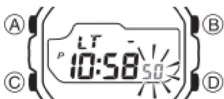
1. In the Timekeeping Mode, hold down (A) until the seconds start to flash, which indicates the setting screen.
