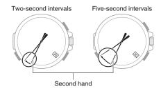
Above right figures indicate a lower battery charge.
