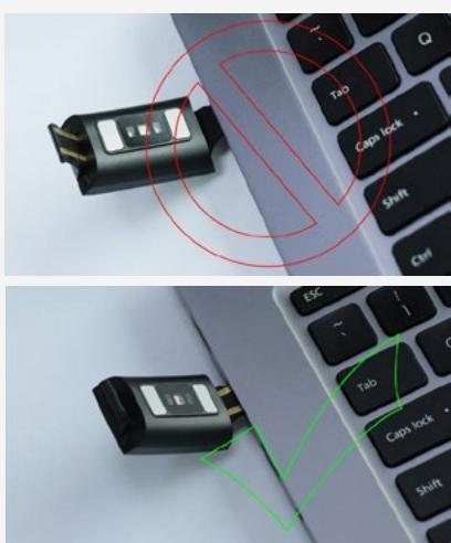
\*Please be aware that the two contacts of charging cannot contact the conductor at the same time, or it may cause the burning of circuit.
